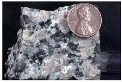
Notice large crystals caused by slow cooling
