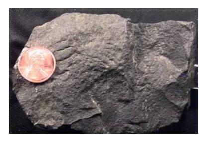
Notice very small crystals caused by fast cooling
